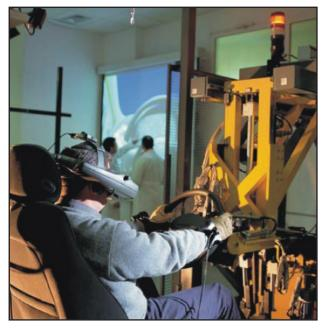
Figure 14. Immersive visualization using seating buck
