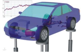
Figure 11. Virtual Suspension Test Rig
