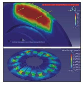
Figure 7. Stress analysis of a rotating brake disk and diaphragm clutch spring
